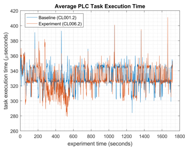
Figure 4-38 - Plots showing the maximum (top) and average (bottom) PLC task execution time during the experiment (left) and during the period of measured impact (right). While the Nessus tool was active, the PLC experienced periods of fluctuating and increased task execution time.
